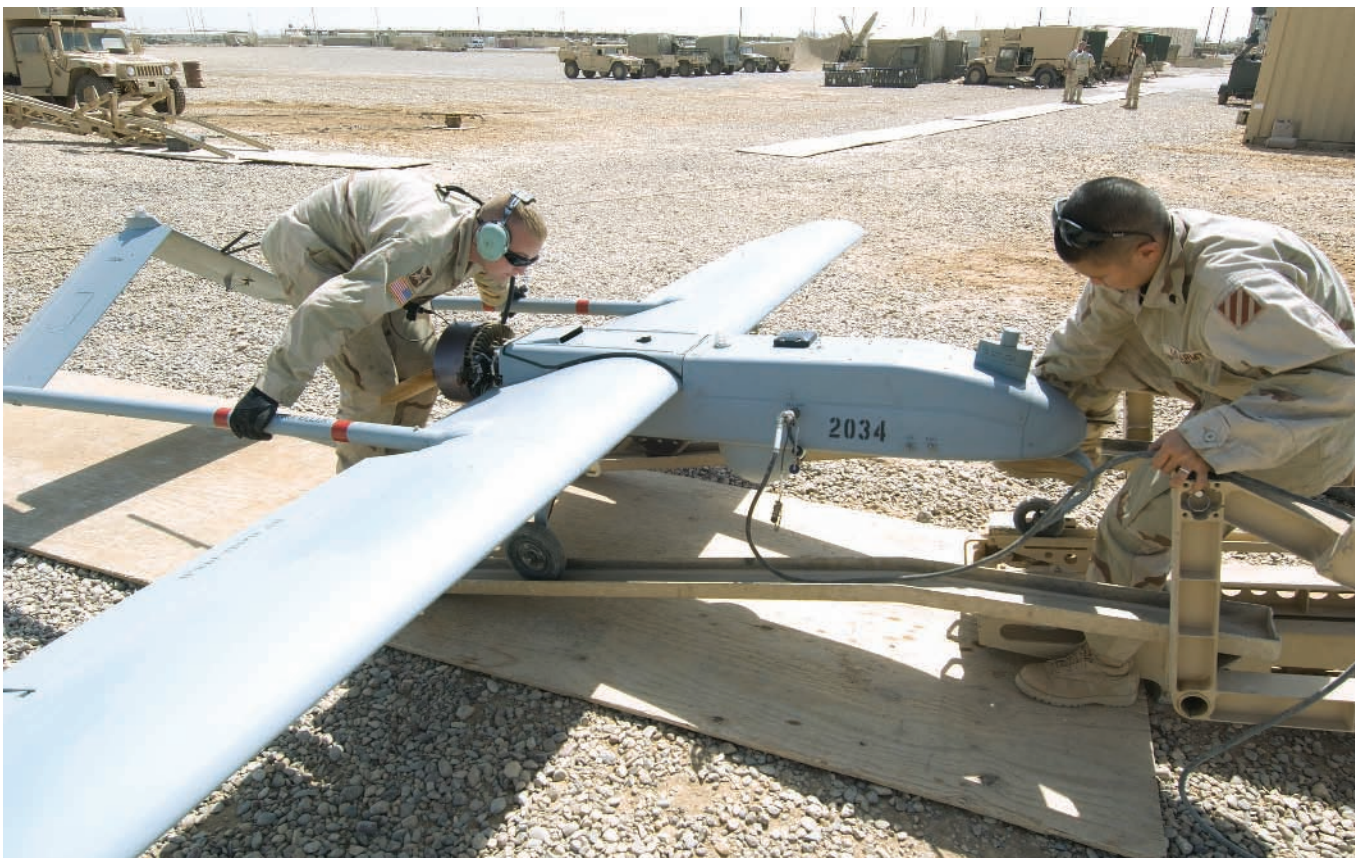
Sgt. Evan Tailford (left) and Spc. Alex Ho move a Shadow TUAV onto the launcher rail to complete preflight preparations.
