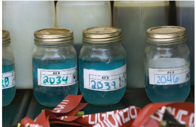
Left, a tactical automated landing system tracking antenna locks onto a TUAV to autonomously bring it in for a landing. Below, fuel samples are taken before every flight as a safety record.
