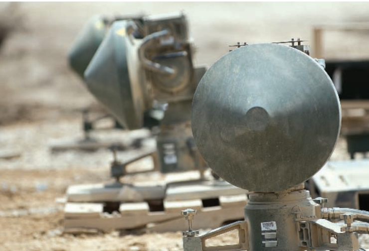
Left, a tactical automated landing system tracking antenna locks onto a TUAV to autonomously bring it in for a landing. Below, fuel samples are taken before every flight as a safety record.
